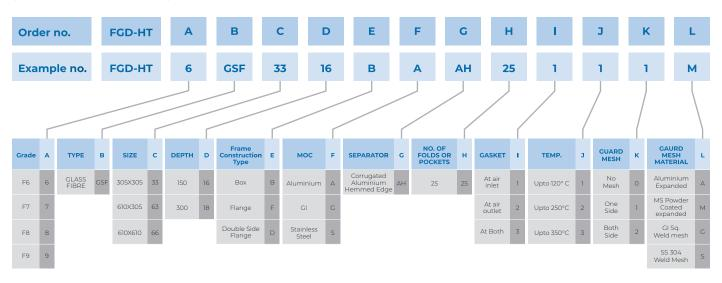
Note: Material of construction Stainless steel is mandatory for 250°C & 350°C.
